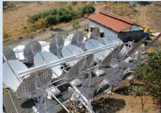
Parabolic Solar reflectors for cooking at Anubhuti School
